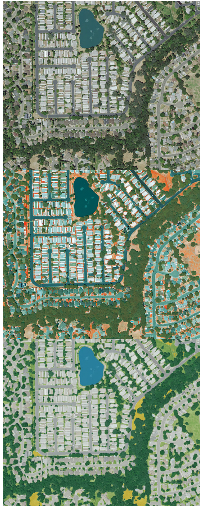
Figure 1. High-resolution aerial imagery (Right) is used to remotely identify existing land cover. Infrared technology delineates living vegetation including tree canopy (Middle). Remote sensing software identifies and maps tree canopy and other land cover (Bottom).
