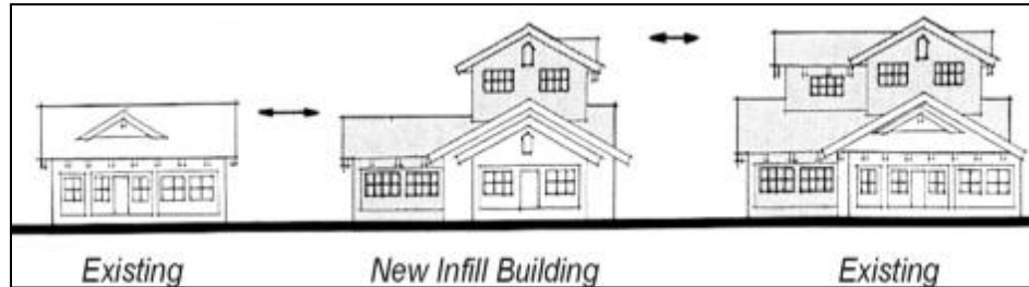
Figure 3-9 - Second Floor Addition Design to Minimize Impact on Smaller House
